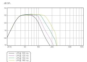
This graph shows the frequency response for a 1-watt swept sine signal in a semi-anechoic environement (2π), measured at 3 m and scaled down at 1 m. In order to provide more precise information for acoustical analysis, a 1/6 octave smoothing has been applied.
