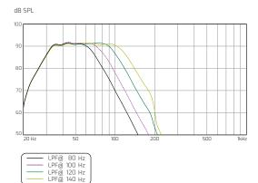
This graph shows the frequency response for a 1-watt swept sine signal in a semi-anechoic environement  $(2\pi)$ , measured at 3 m and scaled down at 1 m.
