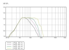
This graph shows the frequency response for a 1-watt swept sine signal in a semi-anechoic environement (2π). measured at 3 m and scaled down at 1 m. In order to provide more precise information for acoustical analysis, a 1/6 octave smoothing has been applied.
