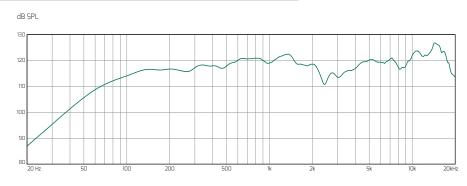
This graph shows the frequency response for a 1-watt swept sine signal in an anechoic environement (4pi), measured at 3 m and scaled down at 1 m.
